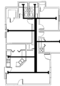
Central Air System
